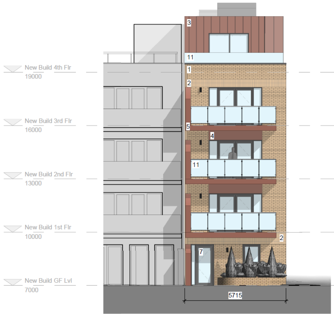
A New Build - North Elevation 1 : 100
